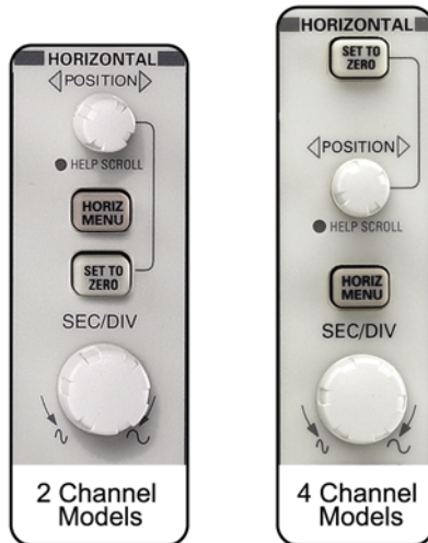
Figure 4.1: The HORIZONTAL control sections
