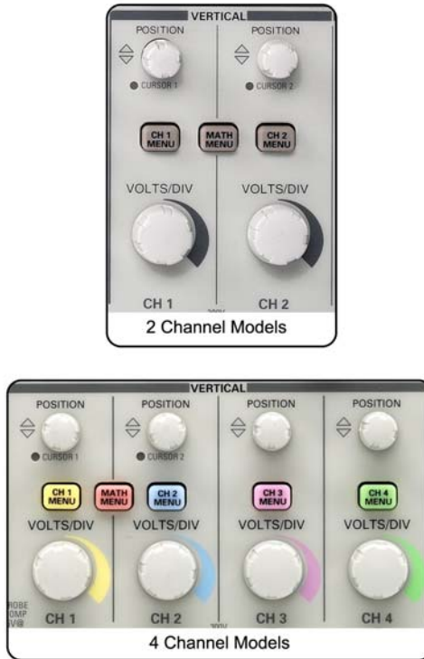
Figure 2.8: TDS1012 and TDS2024 VERTICAL controls
