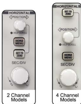
Figure 2.11: TDS1012 and TDS2024 HORIZONTAL controls
